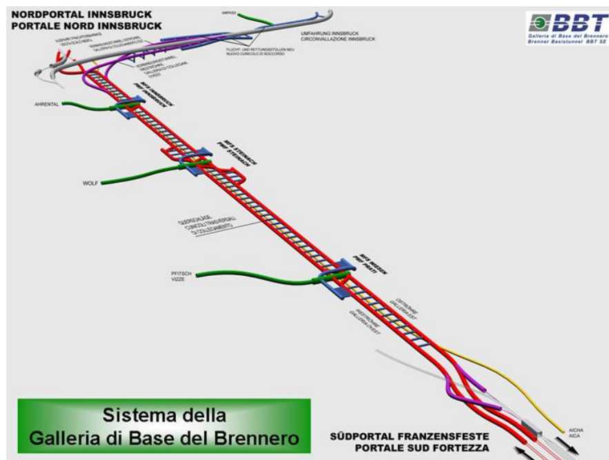
Figure 1.3. Visualisation of the Brenner Basis Tunnel with the pilot gallery (yellow line) between the 2 main galleries (source BBT SE)
