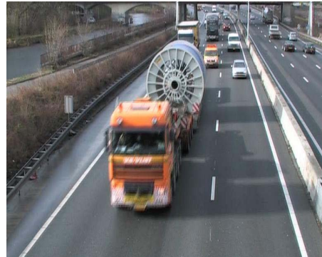
Figure 2: 400kV XLPE drums transported by truck
