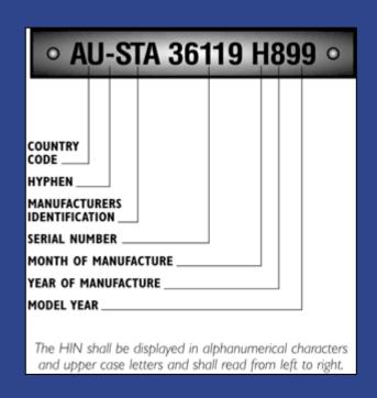
Hull identification changed into craft identification through Directive 2003/44/EC
